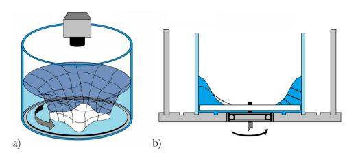
different dispersion relations. Close to the nearly vertical water surface at the center of the cylinder, the flow is dominated by modes referred to as 'centrifugal', whereas gravity wave-like modes are excited simultaneously in the vicinity of the lateral walls. The interactions between these different branches of waves yield the amplification of certain perturbations of coalescent frequencies and wave numbers and the emergence of the polygonal patterns.
